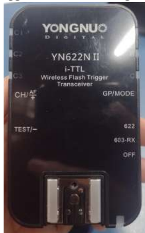
Figura 32-C - Transmissor de flash - Wireless Flash Trigger Transceiver YongNuo
